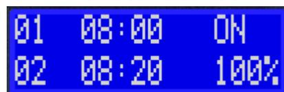
As an example this channel will start up at 8.00 am and raise the lamp brightness up to 100% at 8.20 am.
